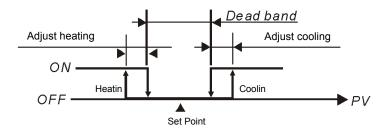
Output of when in PID control mode (Ctrl = PID):
