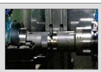
With the principle of relative static, if the spindle speeds are the same and the direction is the same, any two spindles are synchronized by command or feedback. In the synchronous state, one spindle and the other spindle perform the workpiece end-to-end matching and improve processing efficiency, At the same time, avoid machining accuracy errors caused by inaccurate manual clamping. Full-time closed loop synchronization ensures dynamic accuracy.
