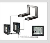
The gantry synchronous axis function can simultaneously perform the displacement of multiple pairs of feed axes without mechanical deviation. The system can quickly process the closed loop control of the synchronous sxis and support the absolute value serial bus encoder such as SSI to improve the performance and efficiency of gantry synchronous control.
