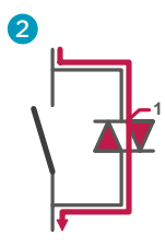
Start: conduction through the semiconductor.
