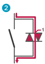
Start: conduction through the semiconductor.
