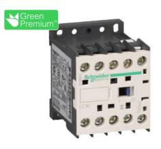
TeSys K contactor , 3P , AC-3 <= 440 V 9 A , 1 NC aux. , 220...230 V AC coil
