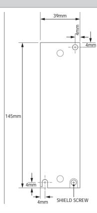
M4 screws should be used in 2 places to mount the MC4N to to an unpainted metal panel.
