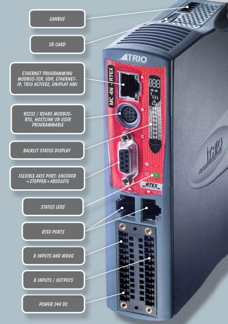
The MC4N-RTEX is dedicated to running remote servo drives via Panasonic's RTEX Real Time EXpress automation bus. It is based on an up-rated version of the 532MHz ARM 11 processor which makes it ideal for high axis count machines or robotic applications.
