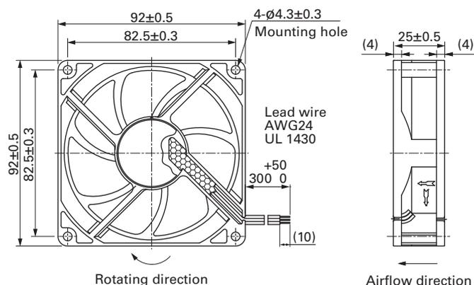
■ Reference Dimensions of Mounting Holes and Vent Opening (unit: mm)
