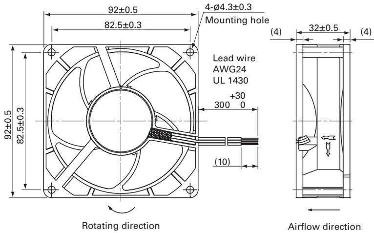
**Reference Dimensions of Mounting Holes and Vent Opening (unit: mm)**
