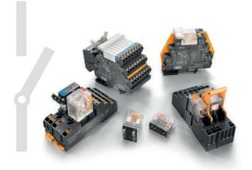
Electromechanical relays are a varied and cost-effective solution for a wide range of switching processes. They can be used for level and power adaptation and form interfaces between control, signalling and regulating equipment and peripherals. In spite of rising raw material prices, they are still very inexpensive and can be easily integrated into a wide variety of circuit types.
