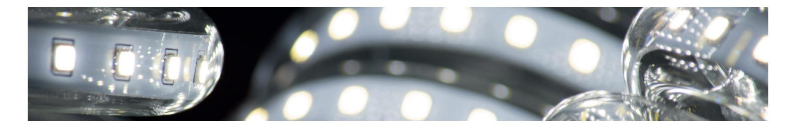
Loads with capacitive load shares, especially LED lamps, place extreme demands on the switching contacts, regardless of the voltage type. They produce extremely high-energy current peaks at the moment of switching on. These can reach over 100 A and weld the contact.
