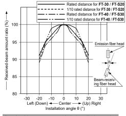
Received-beam amount ratio in Installation angles (FD-30 / FD-40 / FD-S30 / FD-60)
