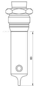
G 1 A hygienic (BCID: A04), PEEK, 83 mm
