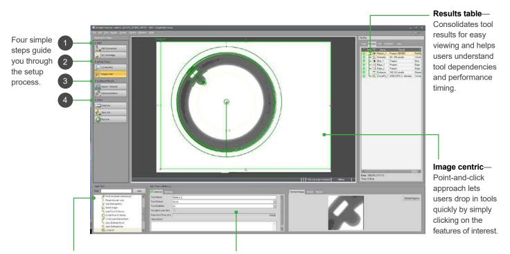
**Tools palette**—Comprehensive set of vision tools for locating, measuring, counting and identifying features, plus math, logic, geometry and graphic display tools.
