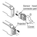
Note: Take care that if the connector is pulled out without pressing the projection, the projection may break. Do not use a sensor head connector whose projection has broken. Furthermore, do not pull by holding the cable, as this can cause a cable-break.
