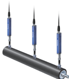
Resin roller eccentricity measurement
