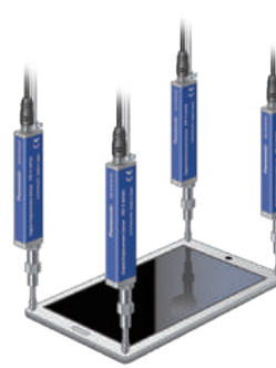
Smartphone flatness measurement
