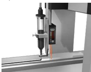
Controlling the height of a dispenser nozzle
