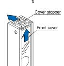
Set the switches of both the emitter and the receiver of Sensor A at '1', and both switches of Sensor B at '2'. The sensors do not function normally at other settings.
