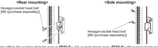
Note: When the number of beam axes is SF4D-F□: 111 or more beam axes, SF4D-H□: 56 or more beam axes, SF4D-A□: 28 or more beam axes, one set is required.
