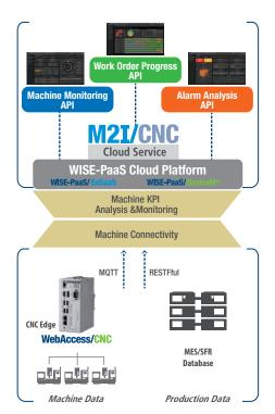
Advantech's M2I/CNC solution consists of two SRPs - CNC Edge and M2I/CNC cloud service - provides comprehensive functions, including real-time machine monitoring, Overall Equipment Effectiveness (OEE) visualization, and performance and abnormality analysis. This solution enables users to rapidly and conveniently implement CNC machine management.
