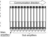
When this product and other products (e.g. fiber sensor amplifiers, pressure sensor controllers, etc.) are connected together in cascade, install those products so that they are in order of Group A, B, D and C as shown in the right figure. This product is included in Group D.
