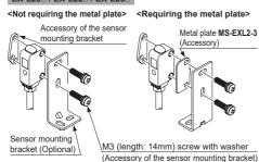
In case not using the metal plate MS-EXL2-□ (accessory) when mounting this product, work on the mounting hole as the diagram below indicates
